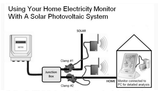
The Home Electricity Monitor is easily used to measure your home's electricity use, along with generated electricity from alternative sources, such as a Solar Photovoltaic system.
